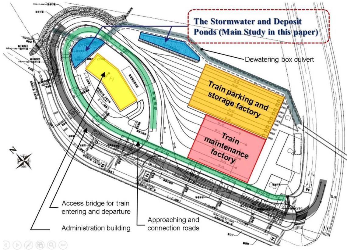
Figure 1 The layout for the depot zone of the ALRMS project
